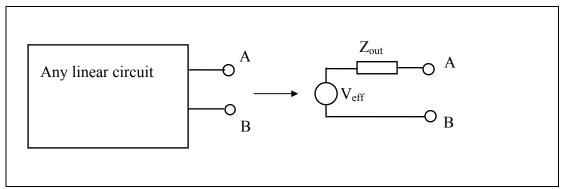
If the circuit is viewed as providing current or voltage to a subsequent stage, the impedance is called the output impedance. (You may have noted that many stereo amplifiers list an **output impedance** of 8 ohms or so.) If the leads are viewed as an input for other signals, the impedance is called the **input impedance**.
