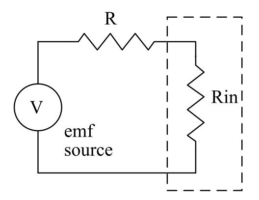
If the circuit being tested also has an output, for example, if the circuit is an amplifier or an oscilloscope or a digital meter, we can use the device output as a monitor of the voltage across  $R_{in}$ . If R is adjustable, we will have the voltage across  $R_{in}$  equal to half V when  $R = R_{in}$ .
