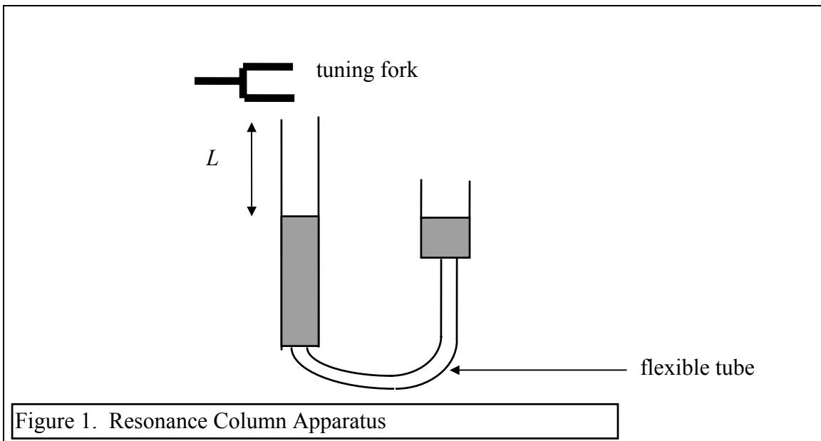
By striking a tuning fork of known frequency on a rubber mallet and placing it close to, but not touching, the mouth of the plastic tube, we can set up forced vibrations of the air
